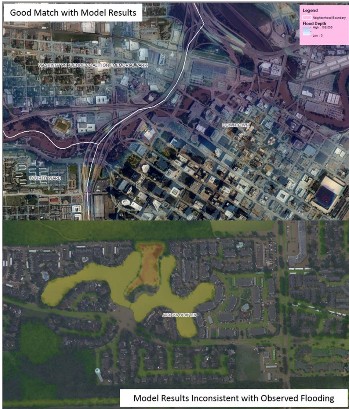
Figure 9. Examples of good and inconsistent matching between model results and observed flooding.
